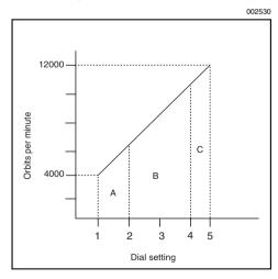
A range: For polishing B range: For finish sanding C range: For regular sanding
